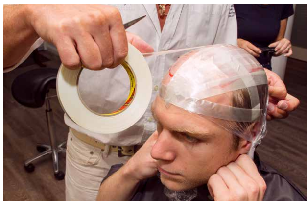
The foil is fixed with a fabric tape (Scotch-895 adhesive tape for stabilising pattern, Art. 4094), lengthwise and crossway.
