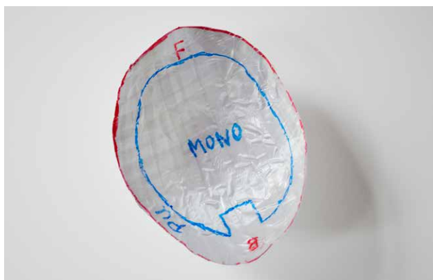
On the pattern can be indicated all information about requested mix of materials. Kindly always indicate F (=Front) as well as B (=Back).
